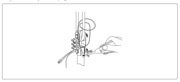
**Step 8**Connect the Connectors from Fan and Receiver. Connect the wires from the receiver to House's Supply Wire. Connect Earth Wire to House Supply Earth Terminal.
