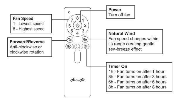
The transmitter & receiver is incorporated with last memory function. This function stores your last setting in memory and the next time you turn on the fan, fan will operate as the last setting.
