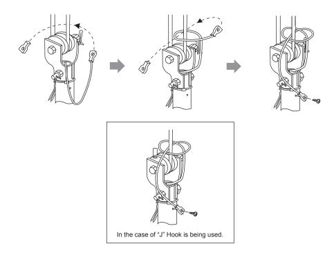
Step 6 - Firmly screw the Safety Wire with spring washer onto the Downrod.
