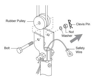
**Step 4** - Remove the Safety Wire screw and spring washer from the Downrod. **IMPORTANT**: Clevis pin MUST be inserted to prevent Nut from loosening.
