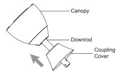
**Step 2** - Route all the wires from the Motor through the Downrod. Fix the Downrod to the coupling with Bolt, Washer, Nut and tighten them firmly then insert the Clevis Pin. **IMPORTANT**: Clevis Pin MUST be inserted to prevent Nut from loosening.
