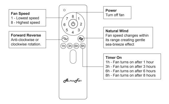
The transmitter & receiver is incorporated with last memory function. This function stores your last setting in memory and the next time you turn on the fan, fan will operate as the last setting.
