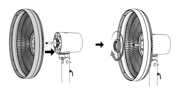
2b. Install the fan blade through the motor shaft vand please make sure the fan blade pin slot is allign with the motor shaft pin. Turn the fan blade lock nut counterclockwise to tighten the nut.
