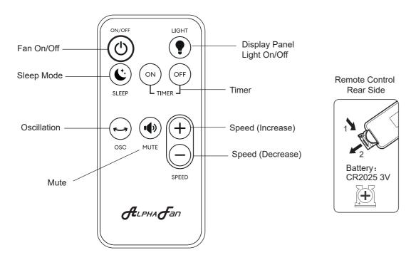
Fan On/Off: Press once to turn On/Off the fan.
